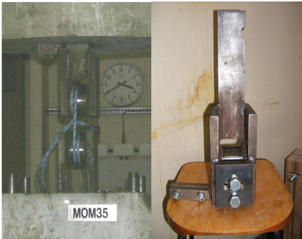
Figure 2 - Test rig set up and shackle assembly
